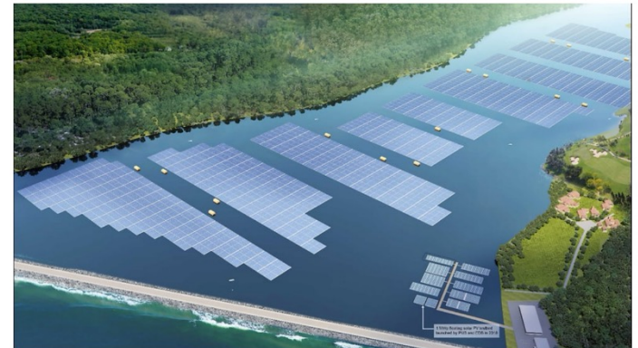
Artist impression of the upcoming 60MWp floating solar system on Tengeh Reservoir. (Photo: PUB/Sembcorp)
