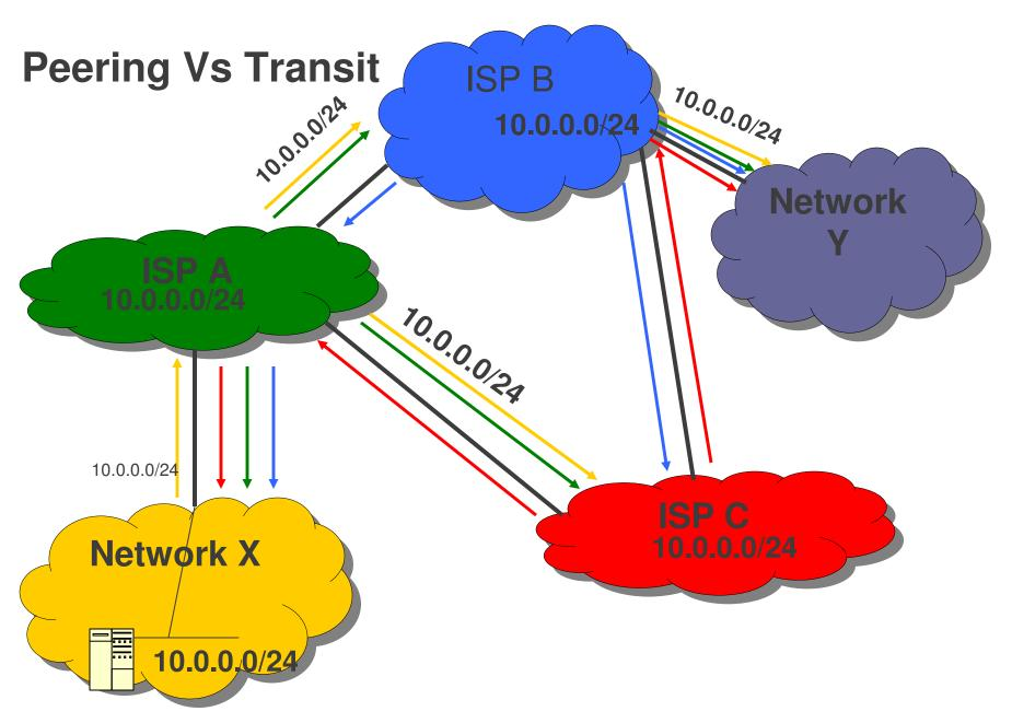
X is a transit customer of ISP A, Y is a transit customer of B. As a transit customer, X announces 10.0.0.0/24 to ISP A. ISP A, B and C peer with each other. Full Mesh at the Tier 1 level required
