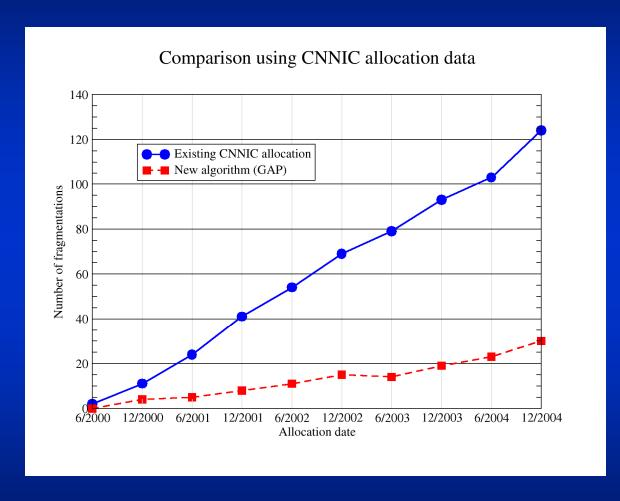
Fragmentation is reduced from 124 to 30 using GAP compared to existing allocation
