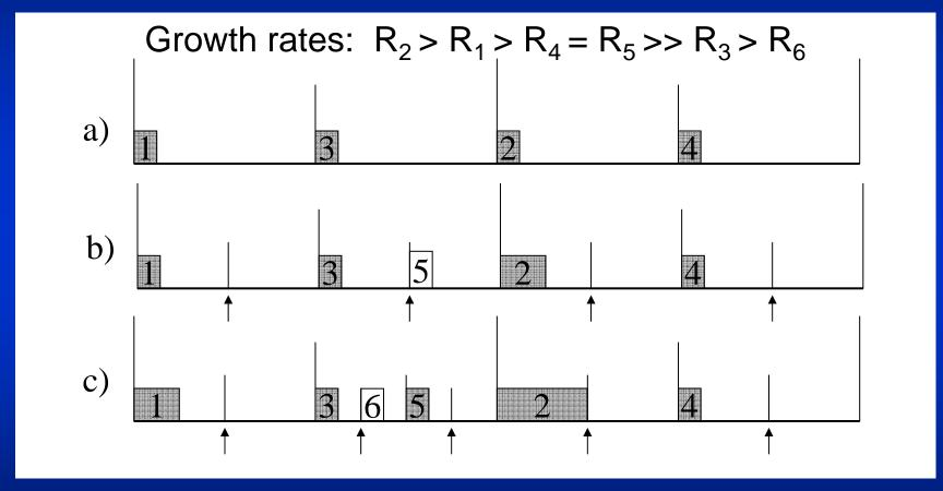
Allocate addresses according to growth-rates.
