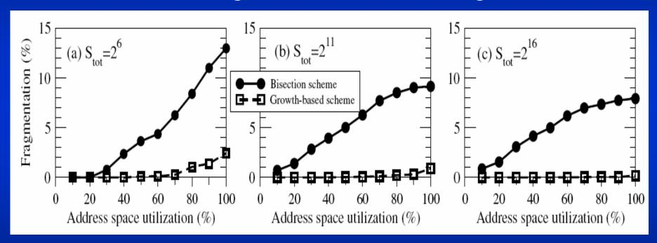
GAP dramatically reduces fragmentation compared to bisection scheme for any percentage of address space utilization.
