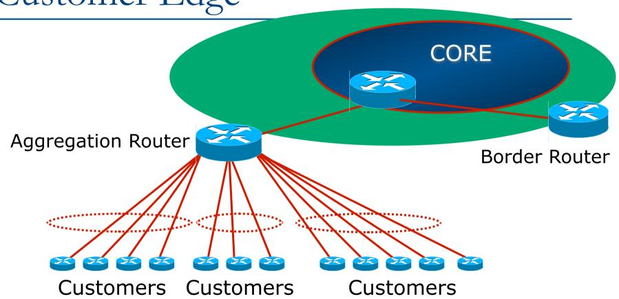
Communities set at the aggregation router where the prefix is injected into the ISP's iBGP
